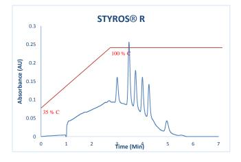
The linear velocity in a narrow bore column at 0.3 ml/min of volumetric flow is around 520 cm/hr in an empty column. Therefore, these compounds are adsorbed regardless of the shear force at such linear velocity.
