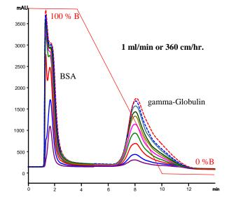
The column is run at volumetric flow rates of 1 and 2 ml/min. The linear velocities are 360 and 720 cm/hr. respectively.
