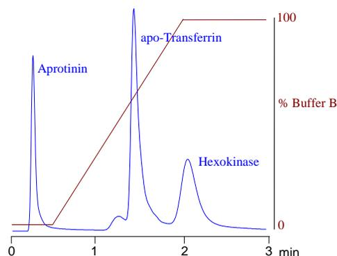
Mixture of Aprotinin, apo-Transferrin and Hexokinase, run at 3 ml/min (1,100 cm/hr) on a 4.6 x 50 mm **STYROS™ DEAE** column
