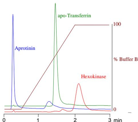
Chromatograms of Aprotinin, apo-Transferrin and Hexokinase, run at 3 ml/min (1,100 cm/hr) on a 4.6 x 50 mm **STYROS™ DEAE** column.
